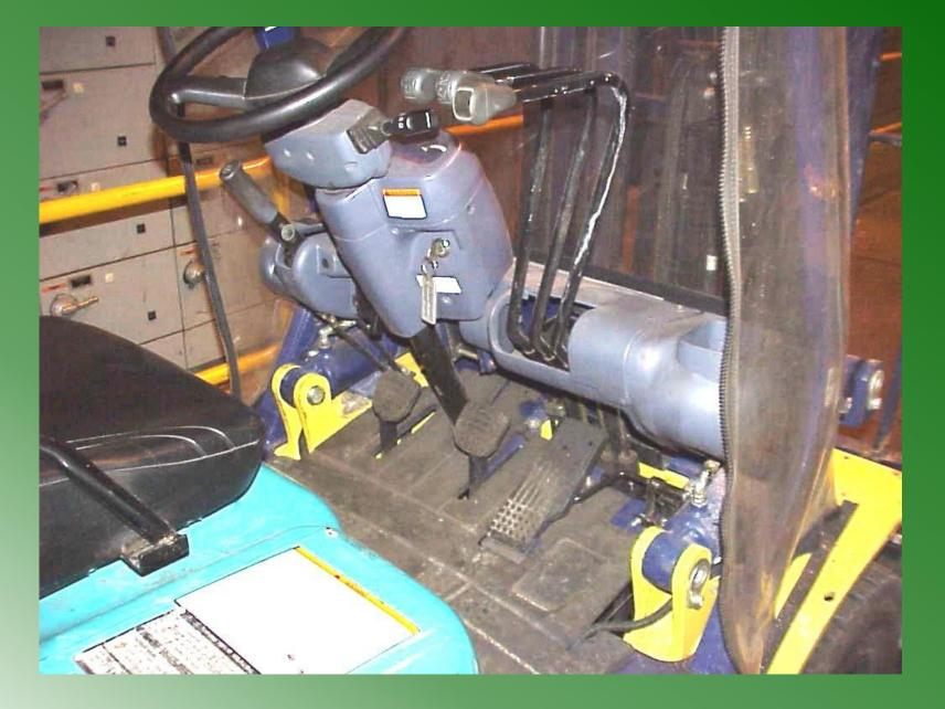
Lower — Tilt Forward — Lift Lever Tilt Lever **Forward Forward** Raise — Tilt Backward Lift Lever Tilt Lever Back **Back**
