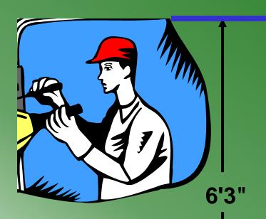
The minimum headroom of working spaces about service equipment, switchboards, panelboards, or motor control centers shall be 6 feet 3 inches
