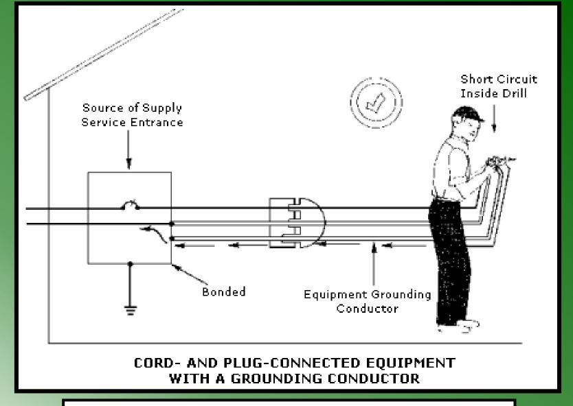
Note that properly bonded conduit and associated metal enclosures can also serve as a grounding conductor.
