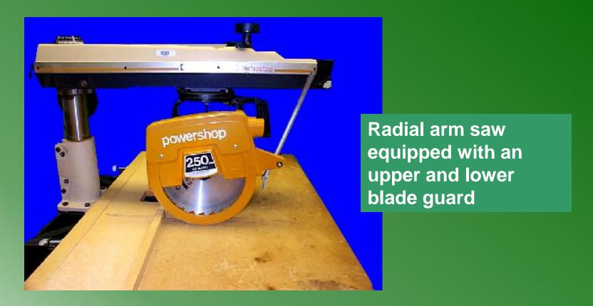
Guard to prevent the operator from coming in contact the the rotating blade
