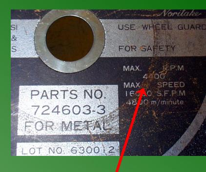
Ensure the spindle speed doesn't exceed the maximum speed marked on the wheel
