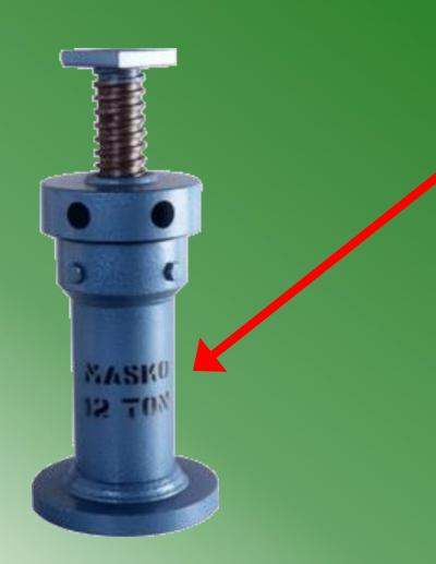
The manufacturer's rated capacity must be marked on all jacks and must not be exceeded
