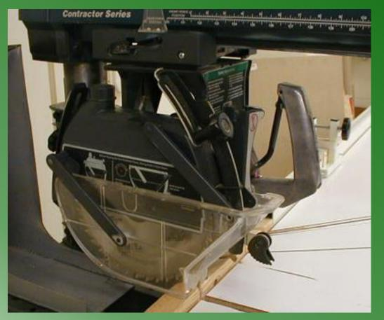
This shows a radial arm saw equipped with proper point of operation guards
