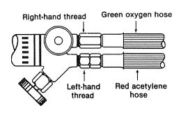
When parallel sections of oxygen and fuel gas hose are taped together, not more than 4 inches out of 12 inches shall be covered by tape.
